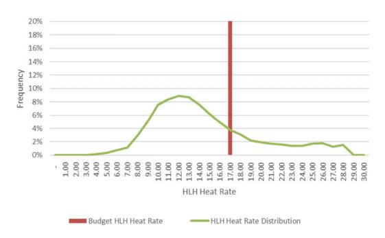
FIGURE 24: STOCHASTIC MODEL OUTPUT: 2022 HLH HEAT RATE DISTRIBUTION
