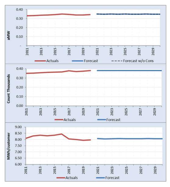
Figure 5-10 – Unmetered Flats forecast of retail load, customers and usage per customer
