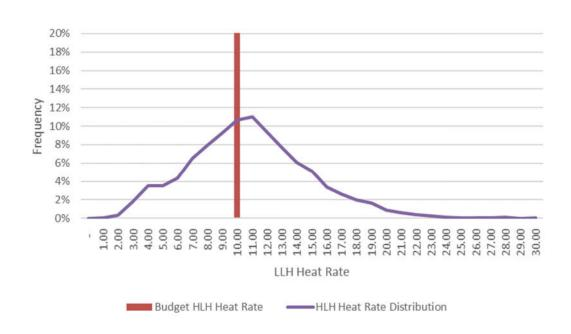
FIGURE 25: STOCHASTIC MODEL OUTPUT: 2022 LLH HEAT RATE DISTRIBUTION
