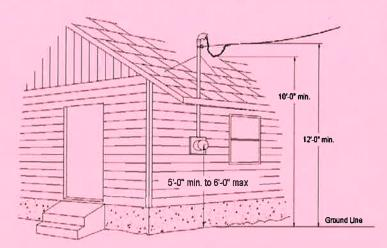
The mast used for attachment of the service drop must be a minimum of a 2-inch rigid steel galvanized conduit, with a suitable attachment to the building to support the weight of the service conductors. Determination of mast height should be made according to applicable service conductor clearances first, then a determination can be made whether mast height will require guying.
